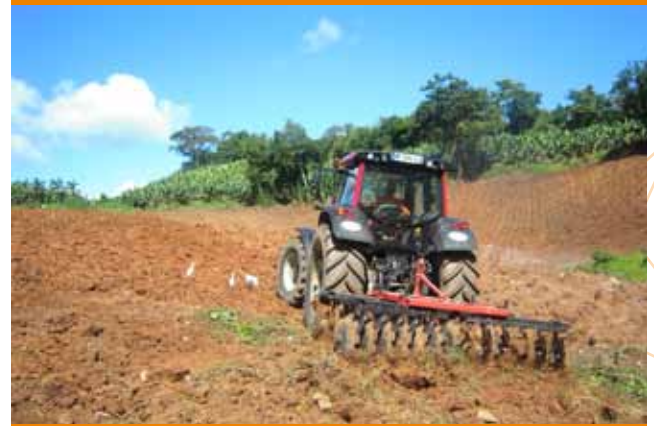
Soil preparation with a disc harrow - Photo IT 2
